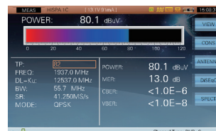
DVB-S/S2 Signal Measurement
