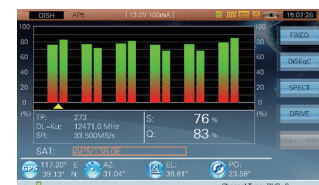
Display Max. 12 Transponder Signals' quality to Align Dish Antenna
