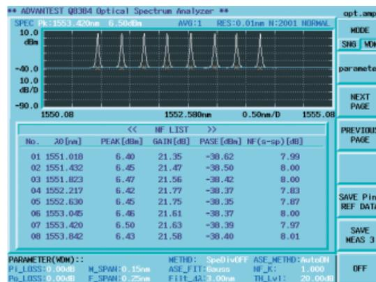
FIG. 7 Measurement Example, DWDM (50 GHz) Noise Figure
