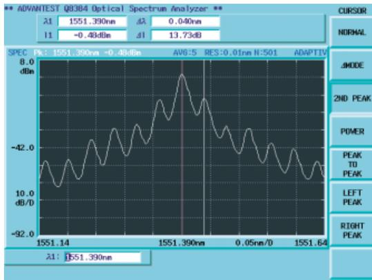
FIG. 2 Sample waveform modulated at 10 Gbps
