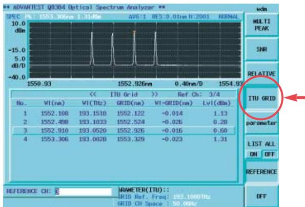
FIG. 10 ITU-T grid display
