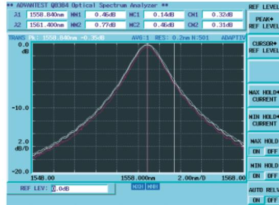
FIG. 21 MAX/MIN/CURRENT simultaneous display
