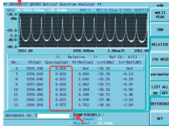
FIG. 3 A measurement example of a Fabry-Perot filter
