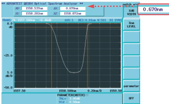
FIG. 14 Notch filter: wavelength width at 3 dB loss
