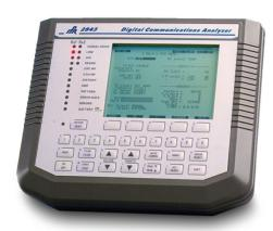
Hand-held, high capability testing for 2 Mbit/s and data line systems and equipment
