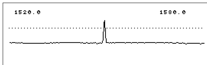
PRBS modulation graph showing raised noise floor.
