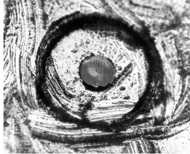
Figure 1-6. Damage from improper cleaning.
